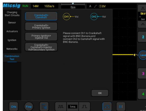
▲ The electronic faults can be complicated, by comparing the collected various waveforms, users judge faults by analyzing the timing and quantitative relationships between waveforms.
