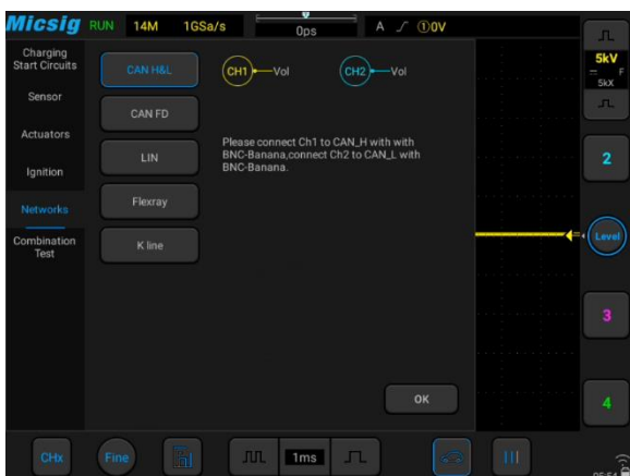
▲ SATO1000 is capable of acquiring and decoding CAN High /CAN Low, CAN FD, LIN, FlexRay, and K line signals, delivers professional Network communication tests on vehicles.
