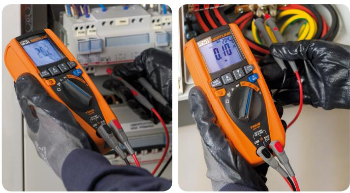
Voltage measurement with test leads.
