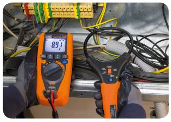
Measurement of current through flexible transducer F3000U.
