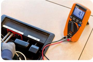
Measurement of voltage harmonics.
